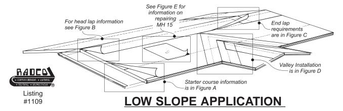
Apply metal eave drip on deck. Apply the starter course of **MH 15**®underlayment, either side up, on the roof deck flush with drip edge of metal eaves strip extending a minimum of 24" into the living space. Fasten this starter course on approximately 18" centers to hold in place.(see Figure A)
