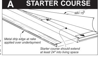
over the starter course and remaining roof using only enough fasteners to hold it in place. Apply metal rake drip edge over the **MH 15**° underlayment if required. (see Figure A)
